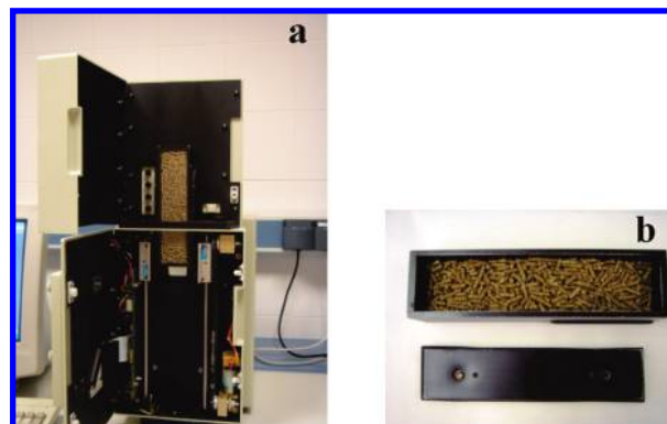
Figure 2. Foss NIRSystems 6500 instrument equipped with transport module and natural cell for unground feedstuffs.
