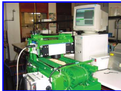
Figure 1. CORONA 45 VIS+NIR instrument on the conveyor belt of the Haldrup stationary module.
